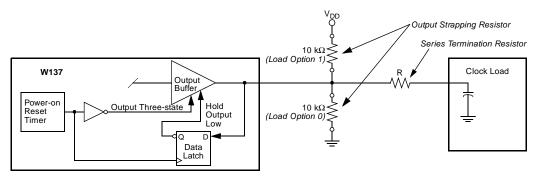
Figure 1. Input Logic Selection Through Resistor Load Option
