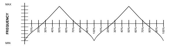
Figure 4. Typical Modulation Profile
