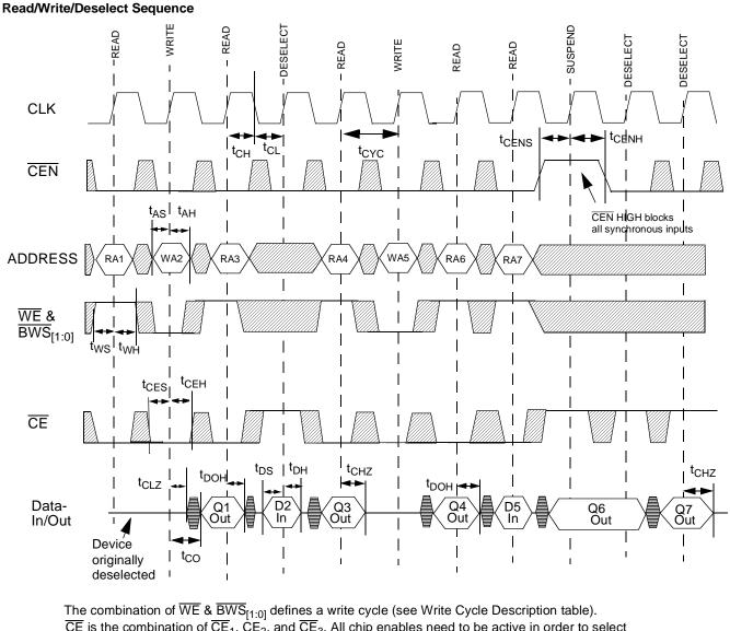
The combination of WE & BWS<sub>[1:0]</sub> defines a write cycle (see Write Cycle Description table).  $\overline{CE}$  is the combination of  $\overline{CE}_1$ ,  $CE_2$ , and  $\overline{CE}_3$ . All chip enables need to be active in order to select the device. Any chip enable can deselect the device. RAx stands for Read Address X, WAx stands for Write Address X, Dx stands for Data-in for location X, Qx stands for Data-out for location X. ADV/LD held LOW.  $\overline{OE}$  held LOW.
