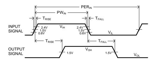
**Timing Diagram For Testing**
