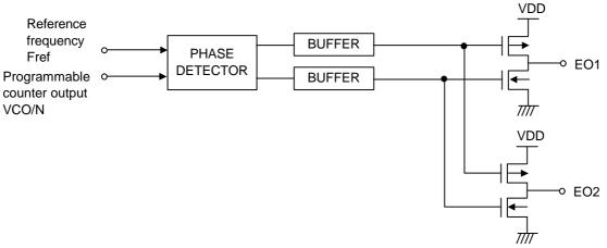
Figure 5-7-8. Phase Detector Circuit Diagram
