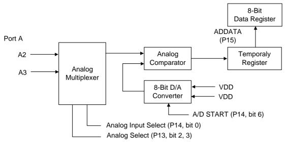
The A/D Converter can be controlled by the three register on the Peripheral File. The function block diagram is shown in Figure 5-7.
