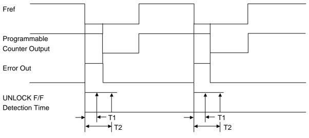
Figure 5-7-2. UNLOCK F/F DETECTION TIME
