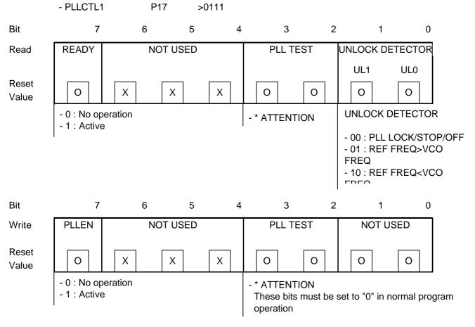
Figure 5-7-5. PLL Control Register
