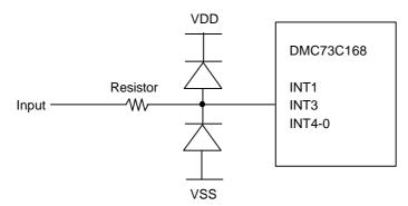
Figure 5-4C Additional Circuitry for External Input
