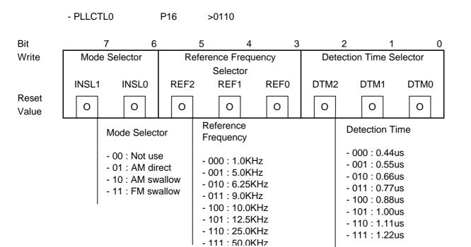
Figure 5-7-1 PLL Control Register
