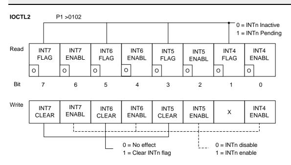
Figure 5-3C I/O Control Register 2 (IOCTL2)
