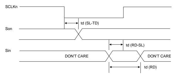
Figure 7.2 AC Characteristics for Serial I/O ports
