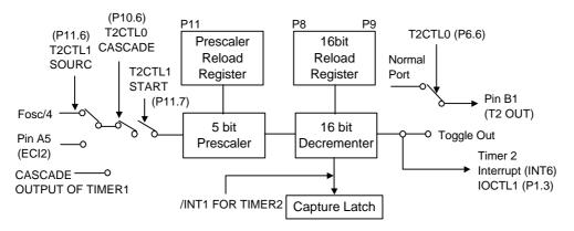
Figure 5-6. Timer 2 Schematic Diagram
