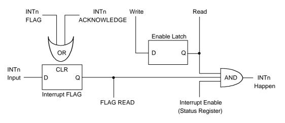
Figure 5-4A-1. Interrupt Logic
