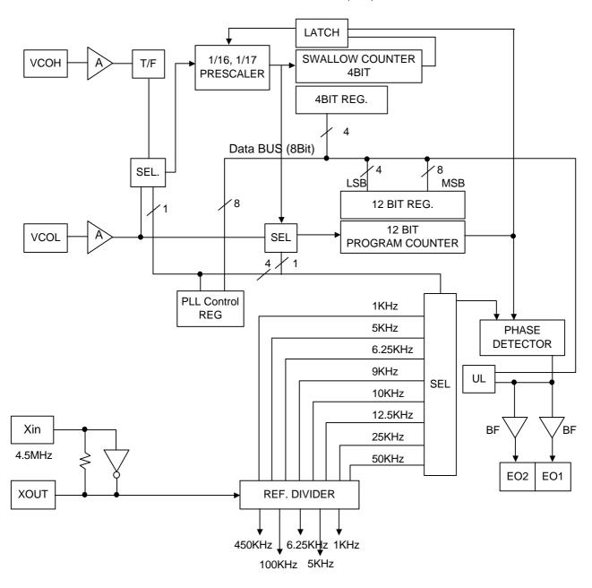
Figure 5-7 PLL Block Diagram
