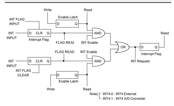
Figure 5-4A-2. Interrupt 4 Logic
