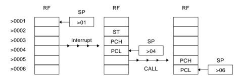
Figure 4.4 Example of Stack Initialization in the Register File
