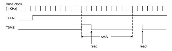
T250MS, T125MS, T100MS, T5MS : Interval timer flag bits.
