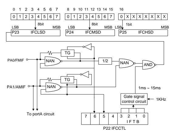
Figure 5-8-1. Configuration of IF counter
