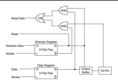
Figure 5-1. Bidirectional I/O Logic
