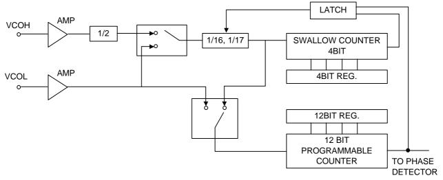
Figure 5-7-7. Circuit Diagram of Programmable Divider
