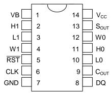
14-Pin DIP (300-mil) See Mech. Drawings Section
