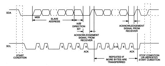
Figure 6 details how data transfer is accomplished on the two-wire bus. Depending upon the state of the  $R/\overline{W}$  bit, two types of data transfer are possible:
