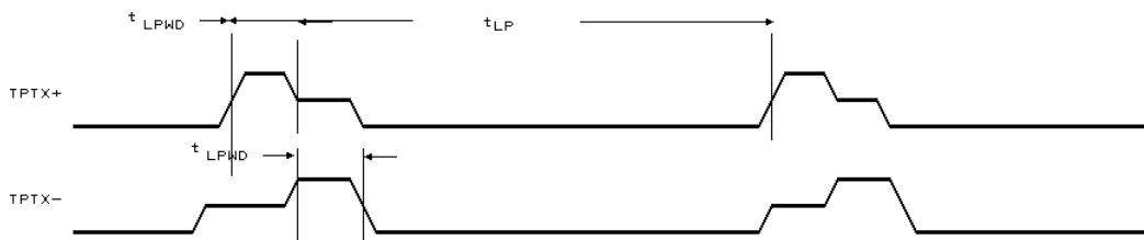
Transmitted Link Integrity Pulse Timing
