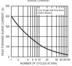
FIG. 1 - MAXIMUM NON-REPETITIVE FORWARD SURGE CURRENT
