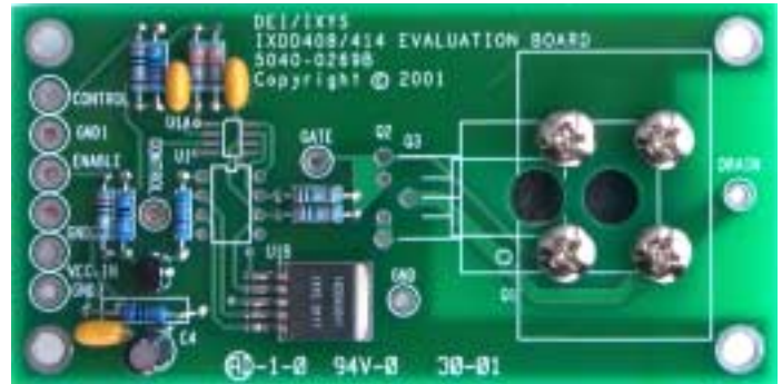
Figure 1 - EVDD408/EVDD414 Evaluation Board SOT-227 Device Installed For Illustration Purposes Only
