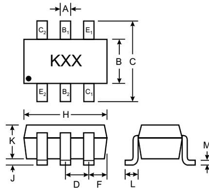
E<sub>1</sub>, B<sub>1</sub>, C<sub>1</sub> = PNP4126 Section
