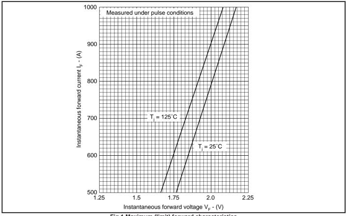
Fig.1 Maximum (limit) forward characteristics
