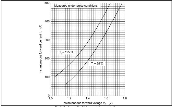
Fig.2 Maximum (limit) forward characteristics
