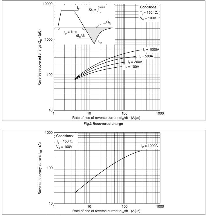
Fig.4 Typical reverse recovery current vs rate of rise of reverse current
