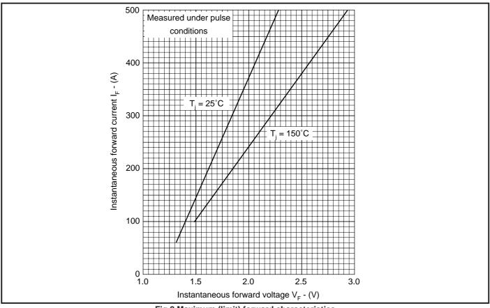
Fig.2 Maximum (limit) forward characteristics
