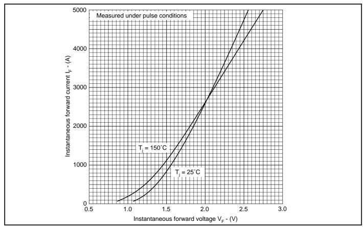
Fig.1 Maximum (limit) forward characteristics
