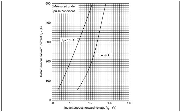
Fig.2 Maximum (limit) forward characteristics
