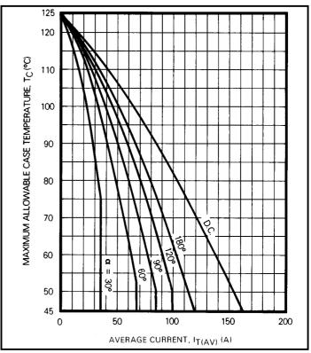
Fig.4 Maximum allowable case temperature for sinusoidal current waveform
