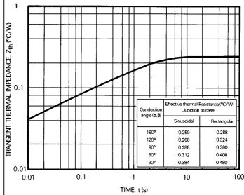
Fig.8 Transient thermal impedance - junction to case
