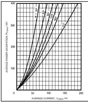
Fig.3 Maximum on-state power dissipation for sinusoidal current waveform
