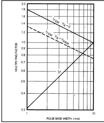
Fig.9 Multiplying factor for non-repetive sub-cycle surge onstate current and  $I^2t$  rating
