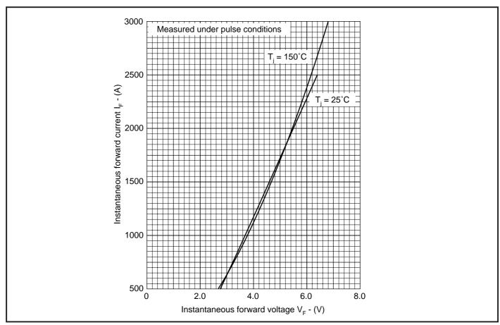
Fig. 1 Maximum (limit) forward characteristics
