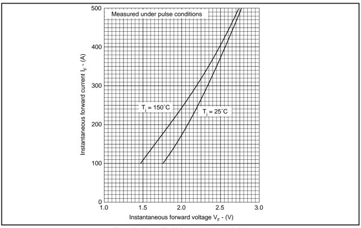
Fig. 2 Maximum (limit) forward characteristics
