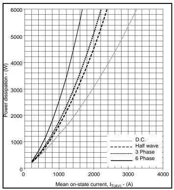
Fig.2 Maximum (limit) on-state characteristics
