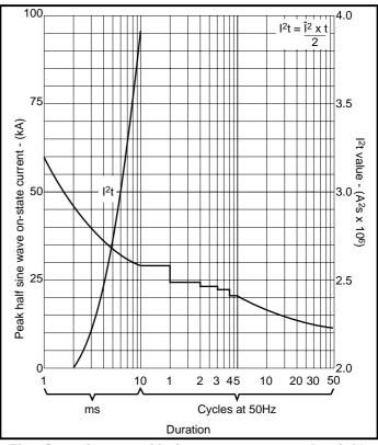
Fig.7 Surge (non-repetitive) on-state current vs time (with 50%  $\rm V_{RSM}$  at  $\rm T_{case}$  = 125°C)
