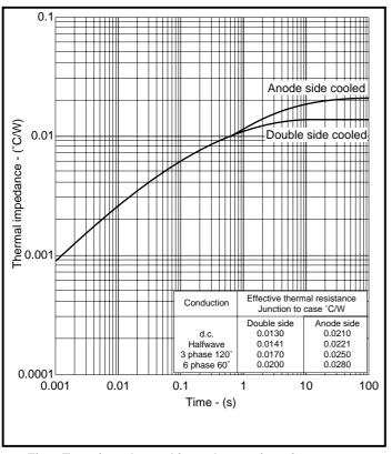
Fig.6 Transient thermal impedance - junction to case
