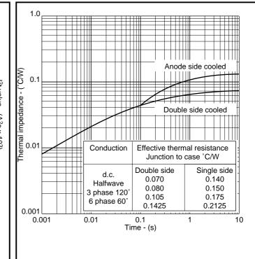
Fig.5 Maximum (limit) transient thermal impedance - junction to case
