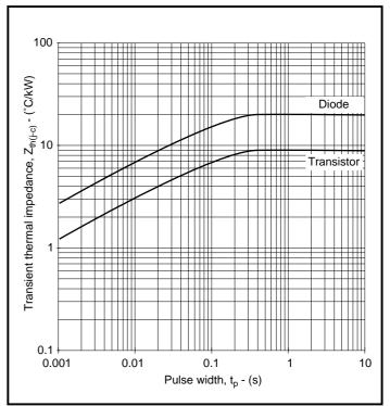
Fig. 10 Transient thermal impedance
