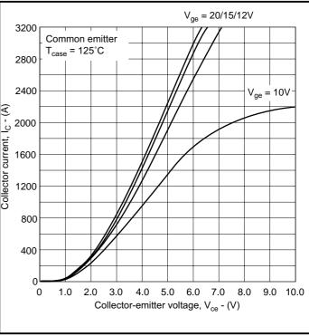
Fig. 3 Typical output characteristics
