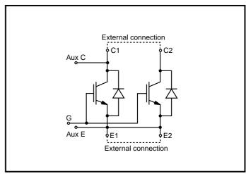
Fig. 1 Single switch circuit diagram
