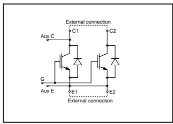
Fig. 1 Single switch circuit diagram
