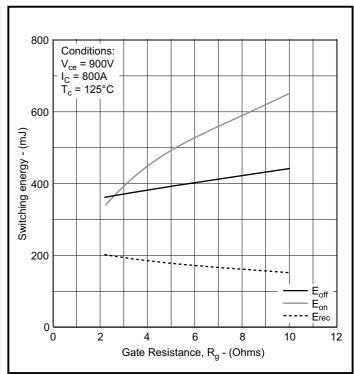
Fig. 6 Typical switching energy vs gate resistance
