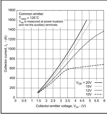
Fig. 3 Typical output characteristics
