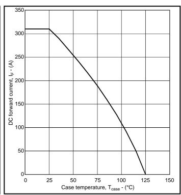
Fig. 6DC current rating vs case temperature
