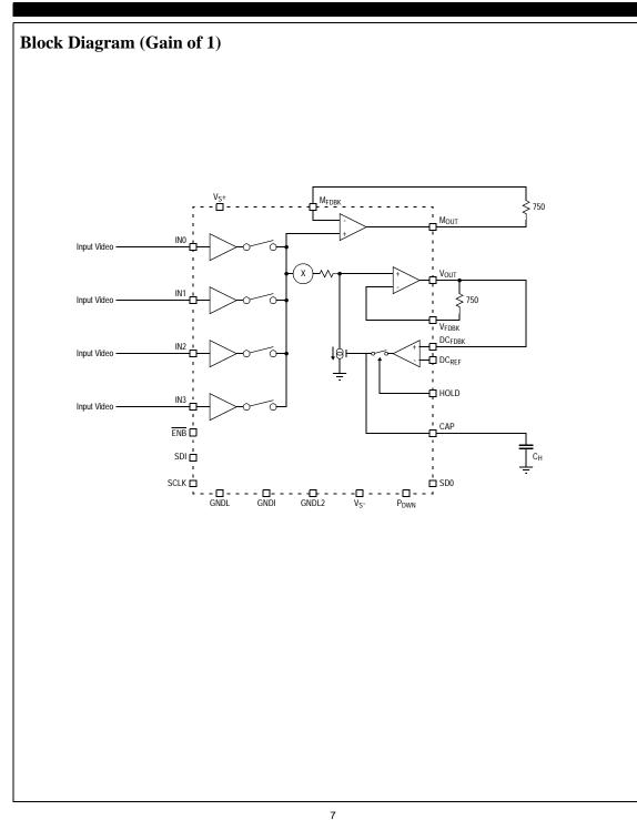
500MHz Video Front End: 4-1 MUX, VGA & DC-Restore
