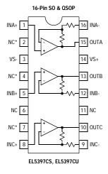
\* This pin must be left disconnected
