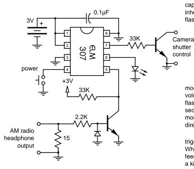
Figure 2. Lightning Detector
