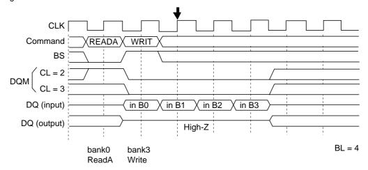
Note: Internal auto-precharge starts at the timing indicated by " lacksquare ".
