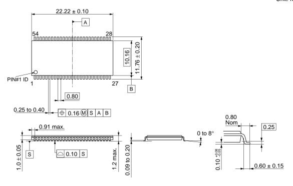
Note: Dimension "A" does not include mold flash, protrusions or gate burrs. Mold flash, protrusions or gate burrs shall not exceed 0.20mm per side.
