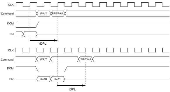
WRITE to PRECHARGE Command Interval (same bank) (BL = 4 (To stop write operation))
