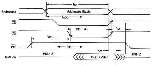
Figure 6. AC Waveforms for Chip/Sector Erase Operations
