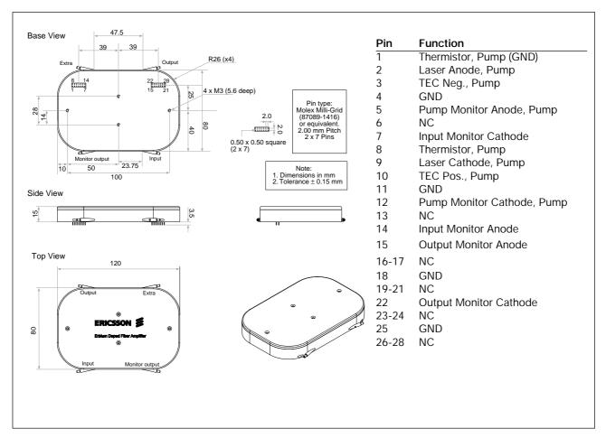
Figure 2. Mechanical Outline Drawing and Pin Connection
