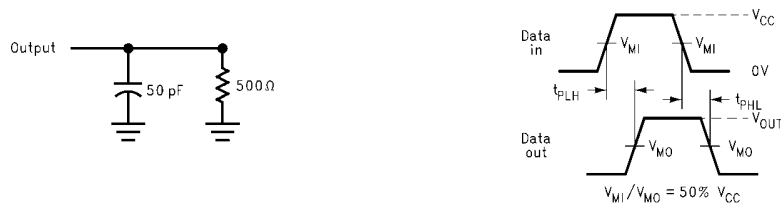
FIGURE 3. t_{PHL} , t_{PLH} Test Load and Waveforms B 1 -B 8 to A 1 -A 8 , C 14 -C 17 to A 14 -A 17 , HLH IN to HLH
