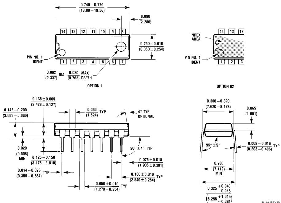
**14-Lead Plastic Dual-In-Line Package (PDIP), JEDEC MS-001, 0.300 Wide
