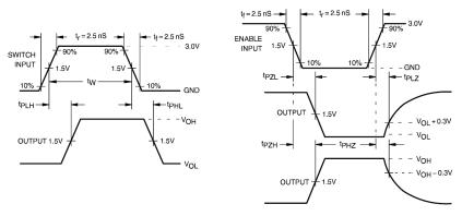
FIGURE 2. AC Waveforms
