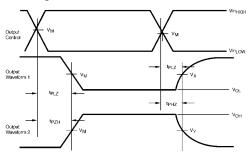
Output Waveform 1 is for an output with internal conditions such that the output is LOW except when disabled by the control output Output Waveforms 2 is for an output with internal conditions such that the output is HIGH except when disabled by the control output
