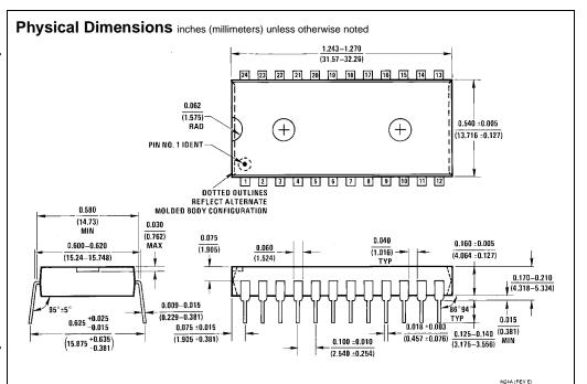
24-Lead Plastic Dual-In-Line Package (PDIP), JEDEC MS-010, 0.600" Wide Package Number N24A
