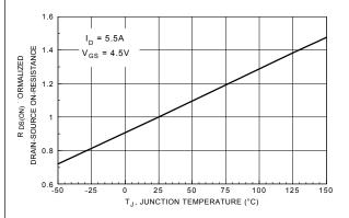
Figure 3. On-Resistance Variation with Temperature.
