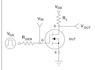
Figure 11. Switching Test Circuit.
