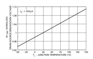
Figure 7. Breakdown Voltage Variation with Temperature.
