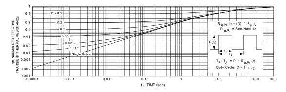
Figure 17. Transient Thermal Response Curve.
