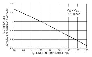
Figure 6. Gate Threshold Variation with Temperature.
