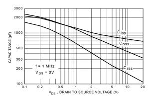
Figure 9. Capacitance Characteristics.
