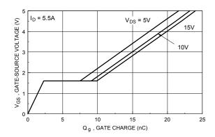
Figure 10. Gate Charge Characteristics.
