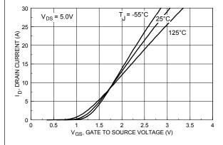
Figure 5. Transfer Characteristics.
