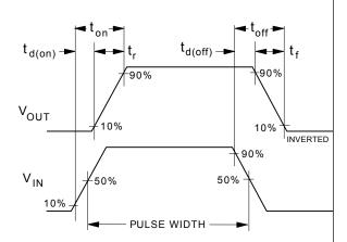
Figure 12. Switching Waveforms.
