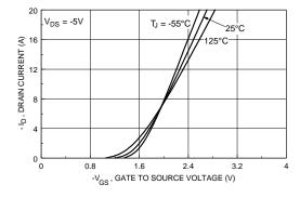
Figure 5.Transfer Characteristics.
