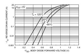
Figure 6. Body Diode Forward Voltage
