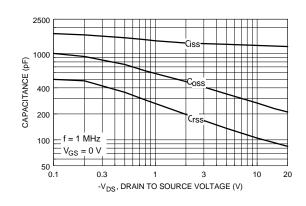
Figure 8. Capacitance Characteristics.
