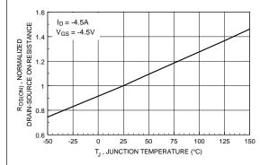
Figure 3. On-Resistance Variation with Temperature.
