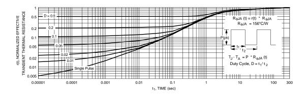
Figure 11. Transient Thermal Response Curve.
