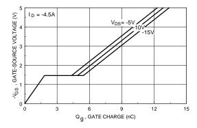
Figure 7. Gate Charge Characteristics.
