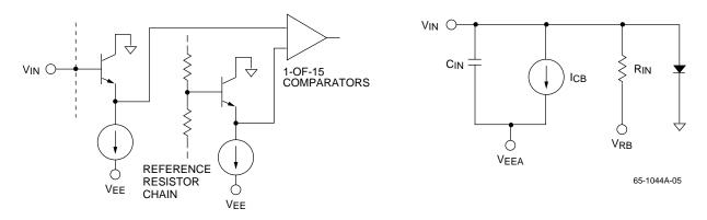
Figure 1. Simplified Analog Input Equivalent Circuit
