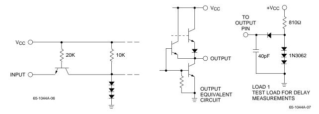
Figure 2. Digital Input Equivalent Circuit
