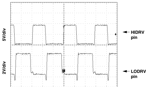
Switching Waveforms, 9A Load
