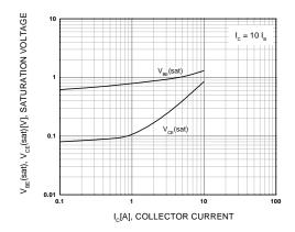
Figure 2. Base-Emitter Saturation Voltage Collector-Emitter Saturation Voltage
