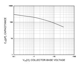
Figure 3. Collector Capacitance
