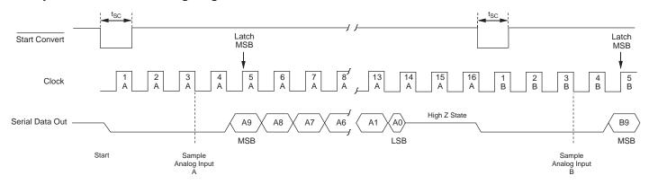
Figure 6 - Free Run Mode Timing Diagram
