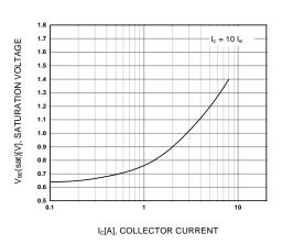
Figure 3. Base-Emitter Saturation Voltage
