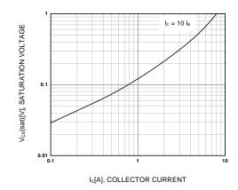
Figure 2. Collector-Emitter Saturation Voltage
