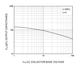
Figure 4. Collector Output Capacitance
