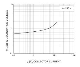
Figure 2. Collector-Emitter Saturation Voltage
