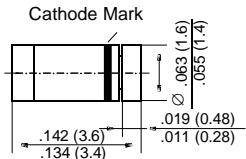
Dimensions are in inches and (millimeters)
