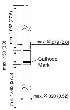
Dimensions are in inches and (millimeters)
