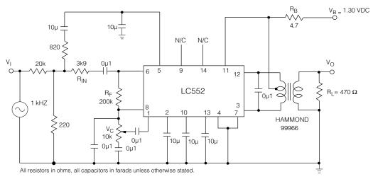
**NOTES:** 1. Test Circuit Amplifier Gain =  $20 \text{ Log}_{10}$  ( $V_O / V_I$ ) + 40 dB
