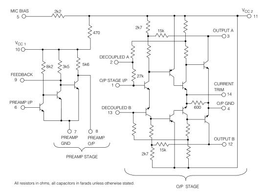
Fig. 2 Functional Schematic Diagram
