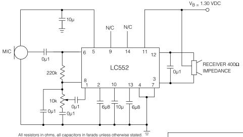
Fig. 3 Typical Hearing Aid Circuit
