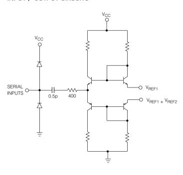
Fig. 1 Input Circuit (Pins 6 and 7)
