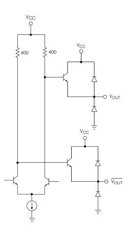
Fig. 2 Output Circuit (Pins 1 and 2)
