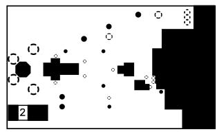
Fig. 32 Ground Layer of EB1504/08 PCB Layout
