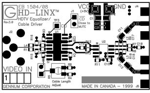
Fig. 30 Top Layer of EB1504/08 PCB Layout
