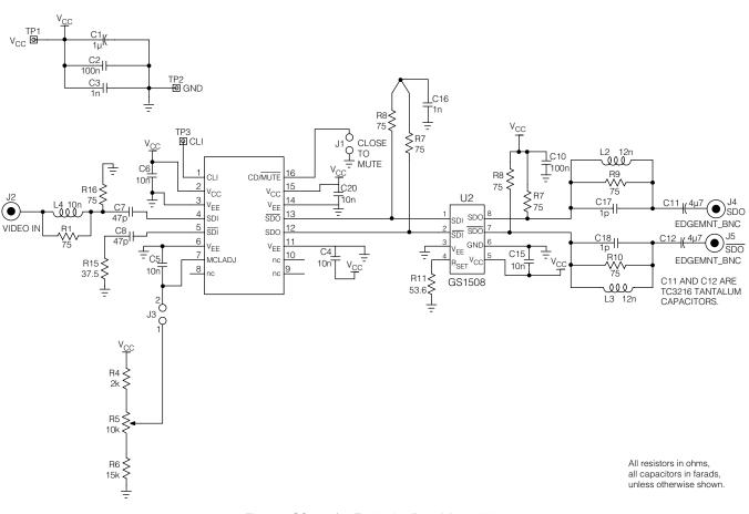
Fig. 29 GS1504/08 Evaluation Board Assembly
