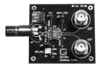
Fig. 28 Photograph of GS1504 Evaluation Board
