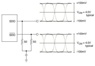
Fig. 21 Typical Output Voltage Levels
