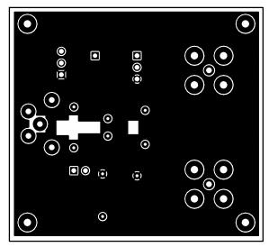
Fig. 27 Power Layer of EB1504 PCB Layout
