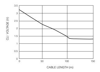
Fig. 20 CLI Voltage vs. Belden 8281 Cable Length
