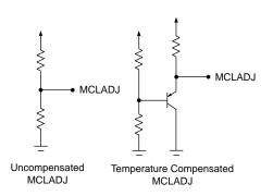
Fig. 10 Temperature Compensation of MCLADJ
