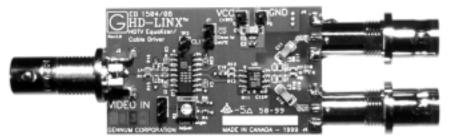
Fig. 34 Photograph of GS1504/GS1508 Evaluation Board
