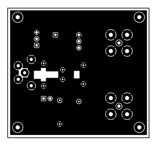
Fig. 25 Ground Layer of EB1504 PCB Layout
