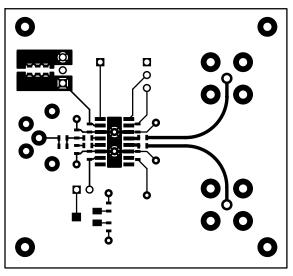
Fig. 24 Top Layer of EB1504 PCB Layout
