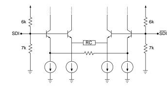
Fig. 2 Input Equivalent Circuit
