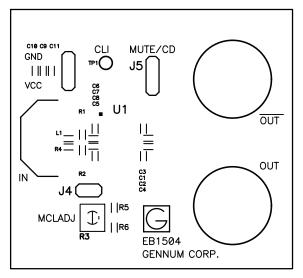
Fig. 23 Silk Screen of EB1504 PCB Layout
