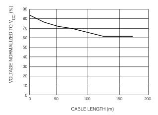
Fig. 12 MCLADJ Input Voltage vs 1694A Cable Length
