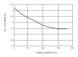
Fig. 19 CLI Voltage vs. Belden 1694A Cable Length
