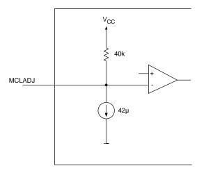
Fig. 3 MCLADJ Equivalent Circuit
