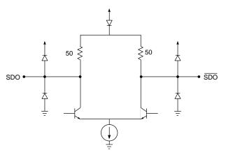
Fig. 4 Output Circuit
