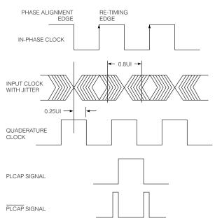
Fig. 20 PLL Circuit Principles
