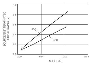
Fig. 23 Signal Swing for Various R<sub>SET</sub> Admittances
