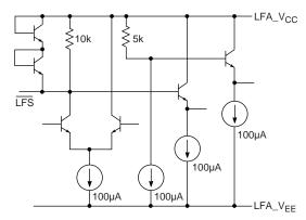
Fig. 6 LFS Input Circuit
