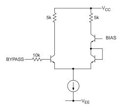
Fig. 13 BYPASS Circuit
