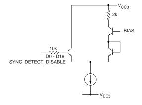
Fig. 10 Data Input and SYNC\_DETECT\_DISABLE Circuit
