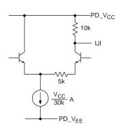
Fig. 8 IJI Output Circuit
