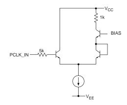
Fig. 11 PCLK\_IN Circuit
