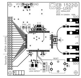
Fig. 28 Top Layer of EB1522 PCB Layout
