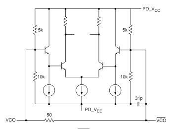
Fig. 1 VCO/VCO Input Circuit
