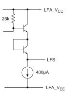
Fig. 5 LFS Output Circuit
