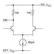
Fig. 2 DM Output Circuit
