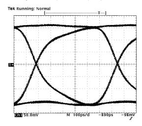
Fig. 25 Compensated Output Eye Waveform
