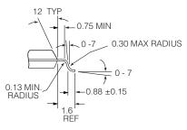
128 pin MQFP All dimensions are in millimetres.
