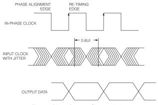
Fig. 16 Phase Detector Characteristics
