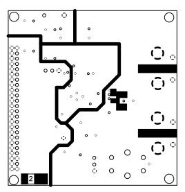
Fig. 29 Ground Layer of EB1522 PCB Layout
