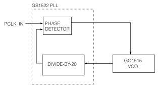
Fig. 15 Phase Lock Loop Frequency Synthesis
