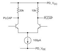
Fig. 3 PLCAP/PLCAP Output Circuit
