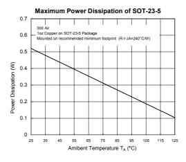
Figure 4 Power Dissipation vs. Temperature
