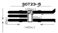
Figure 2. Recommended Minimum Footprint
