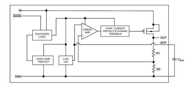
Figure 1. Functional Diagram
