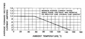
Fig. 3 - MAXIMUM AVERAGE FORWARD CURRENT RATING
