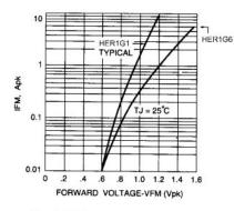
Fig. 2 - FORWARD CHARACTERISTICS
