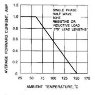
Fig. 3-FORWARD CURRENT DERATING CURVE
