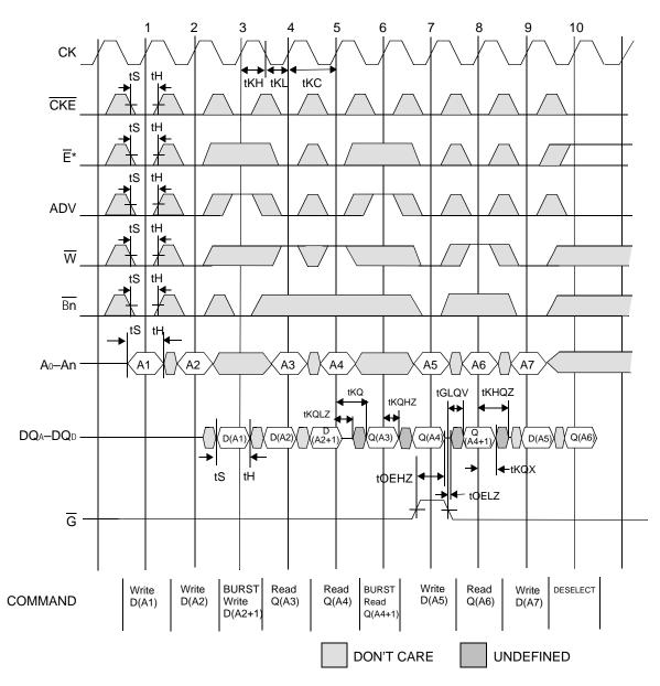
\*Note:  $\overline{E}$  = High (False) if  $\overline{E}_1$  = 1 or  $E_2$  = 0 or  $\overline{E}_3$  = 1
