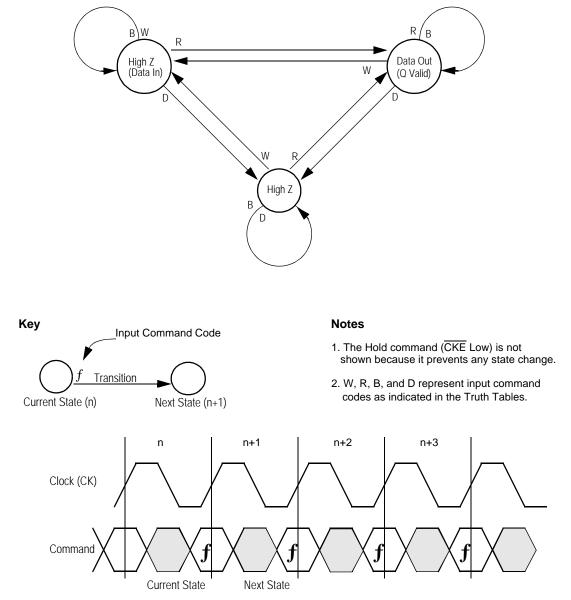
Current State and Next State Definition for: Pipeline and Flow Through Read Write Control State Diagram
