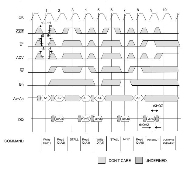
\*Note:  $\overline{E}$  = High (False) if  $\overline{E}_1$  = 1 or  $E_2$  = 0 or  $\overline{E}_3$  = 1
